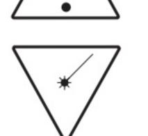
**DANGER:** This symbol is intended to alert the user to the risk of exposure to invisible and hazardous laser radiation if the cover or back is opened the interlock fails or is defeated. Direct exposure to the beam may damage your eyesight.
