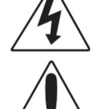
**DANGEROUS VOLTAGE:** The lightning flash with arrowhead symbol within an equilateral triangle is intended to alert the user to the presence of uninsulated dangerous voltage within the product's enclosure that may be of sufficient magnitude to constitute a risk of electric shock to persons.
