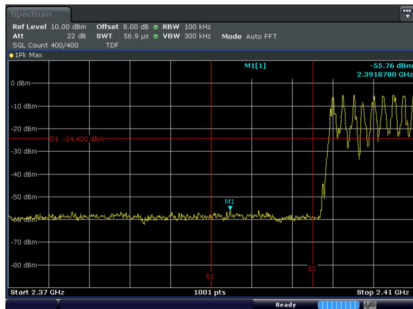
**A.3. Lowest Ch. (2 402 MHz)\_Spurious emissions**
