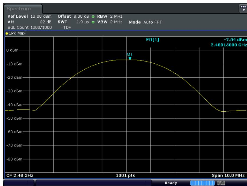
**Test mode : EDR****A. Lowest Ch. (2.402 MHz)**
