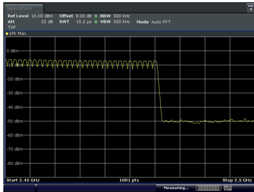
**Test mode : EDR****A. Lowest Band. (Hopping)**
