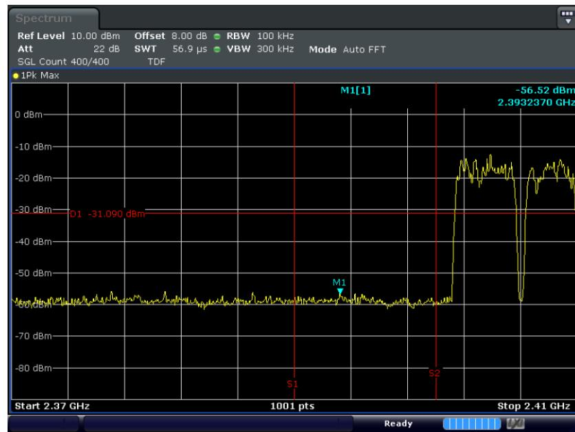
**A.3. Lowest Ch. (2 402 MHz)\_Spurious emissions**
