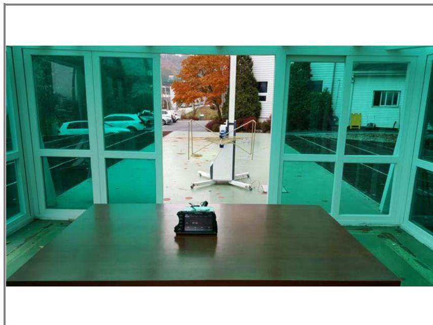
**Photo of radiated spurious emission at above 1 000 □**
