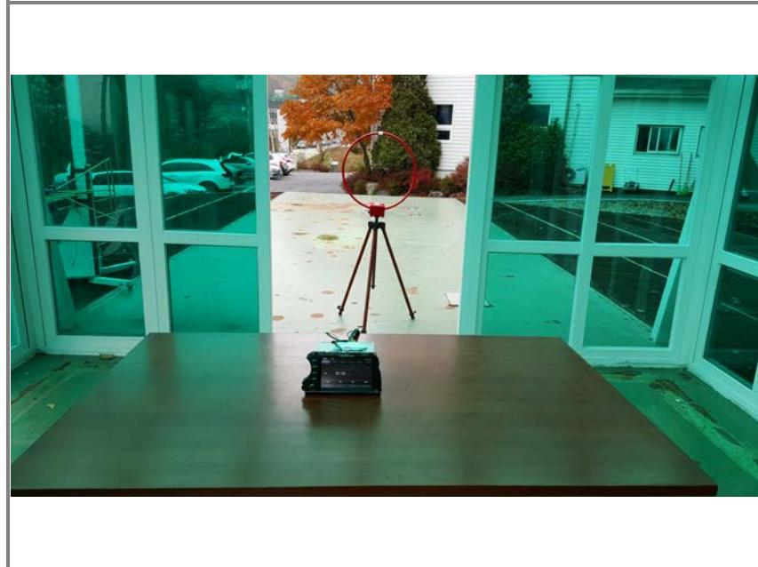
**Photo of radiated spurious emission at 30  $\mu$  ~ 1 000  $\mu$**
