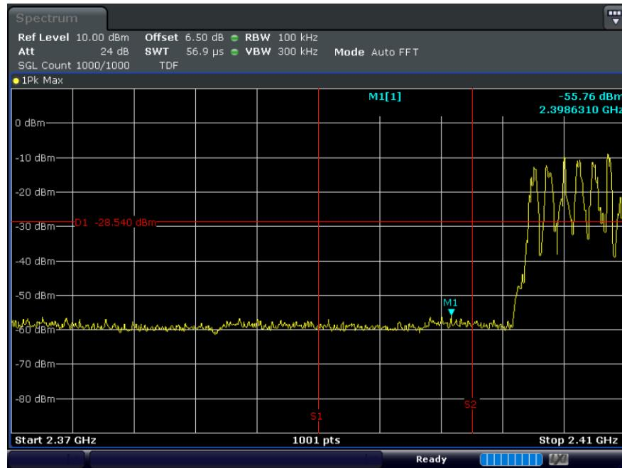
**A.3. Lowest Ch. (2 402 MHz)\_Spurious emissions**
