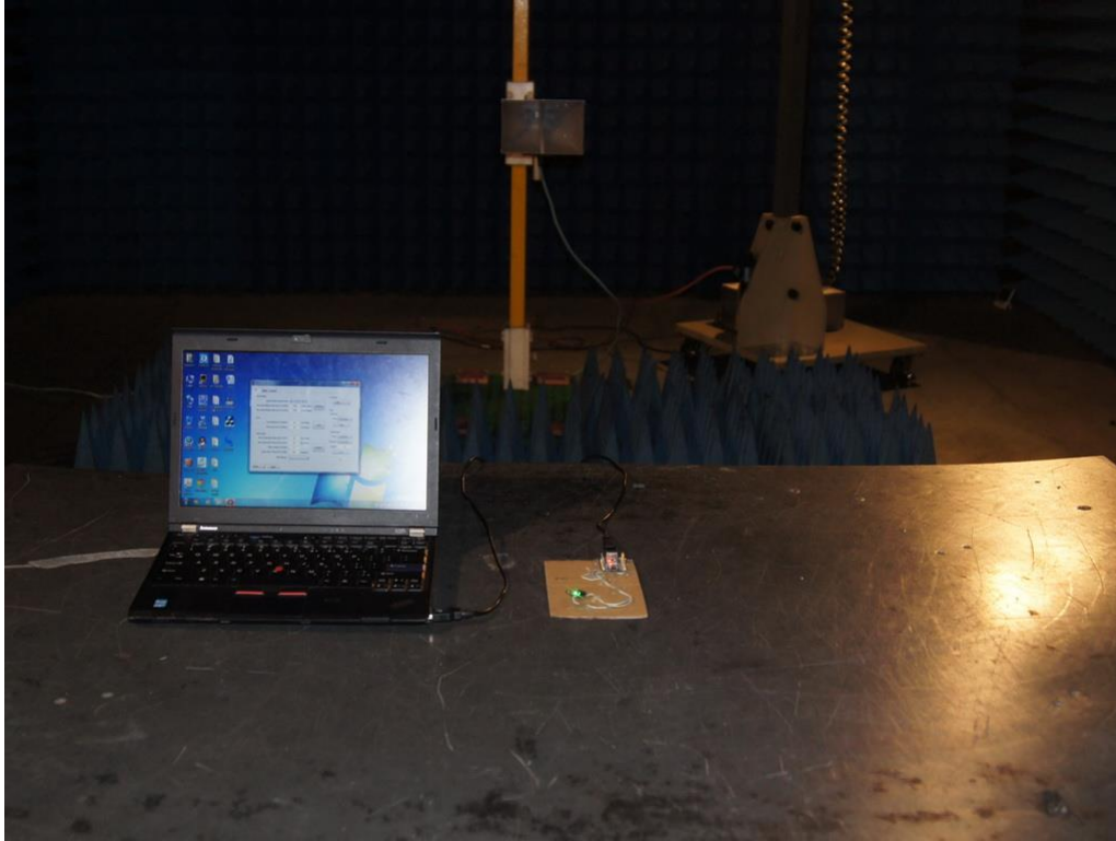
Photograph 4: Set-up for Spurious Emissions (18GHz-26GHz)
