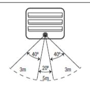
PIR sensor detection distance: 3-5m
