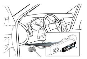
Use the supplied wire taps to wrap the CSM cables on the back of the OBD (see diagram below, points 1 to 3).
