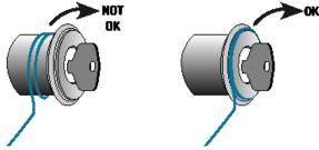
Fix and tape the ring around the ignition, excess cable can be taped together but may not be turned around (one rotation maximum). When using the ring method for installing the CSM, the ring MUST be taped in front of the factory receiver ring. It CAN NOT be on top of, or behind the factory receiver ring. See illustration above. The antenna cable must follow existing steering column cables to avoid rupture while closing the shroud or moving the steering wheel.
