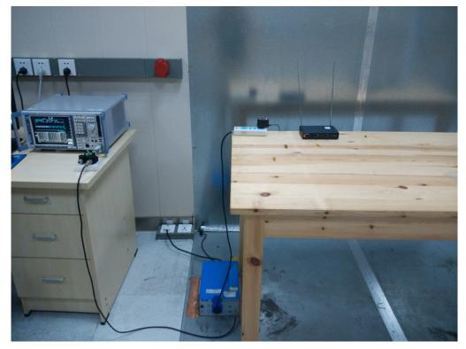
RADIATED EMISSION TEST SETUP
