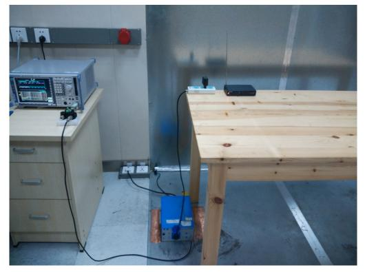
RADIATED EMISSION TEST SETUP
