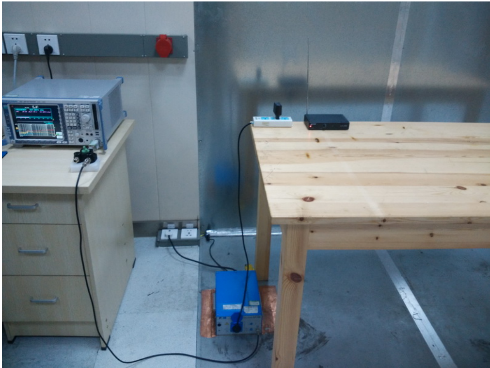
RADIATED EMISSION TEST SETUP
