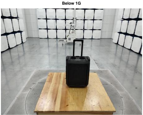
Radiated Emissions Test Setup
