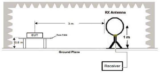
(2) Radiated Emission Test-Up Frequency 30MHz~1GHz
