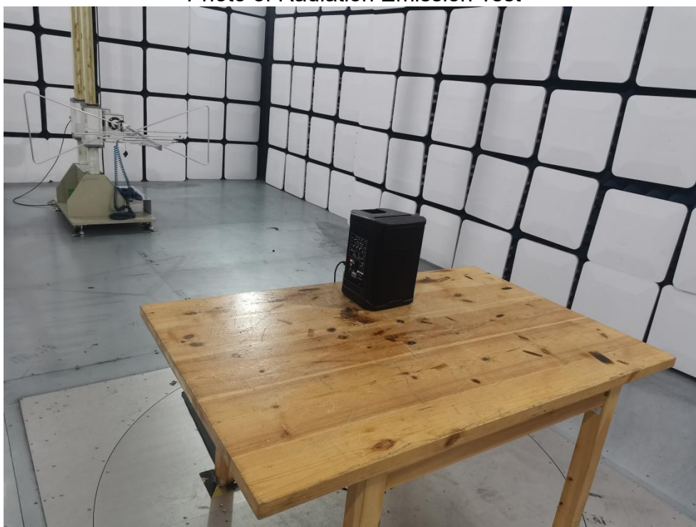
Photo of Radiation Emission Test
