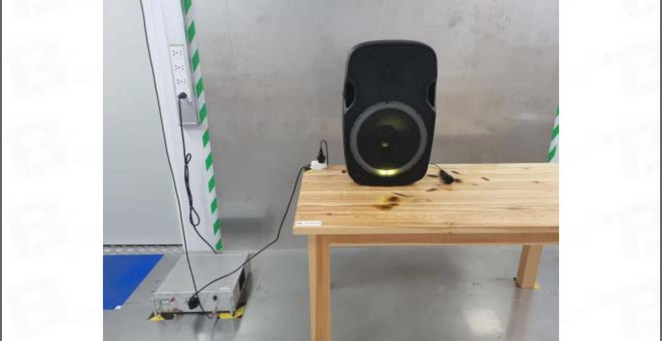
Conducted Emission at AC power line
