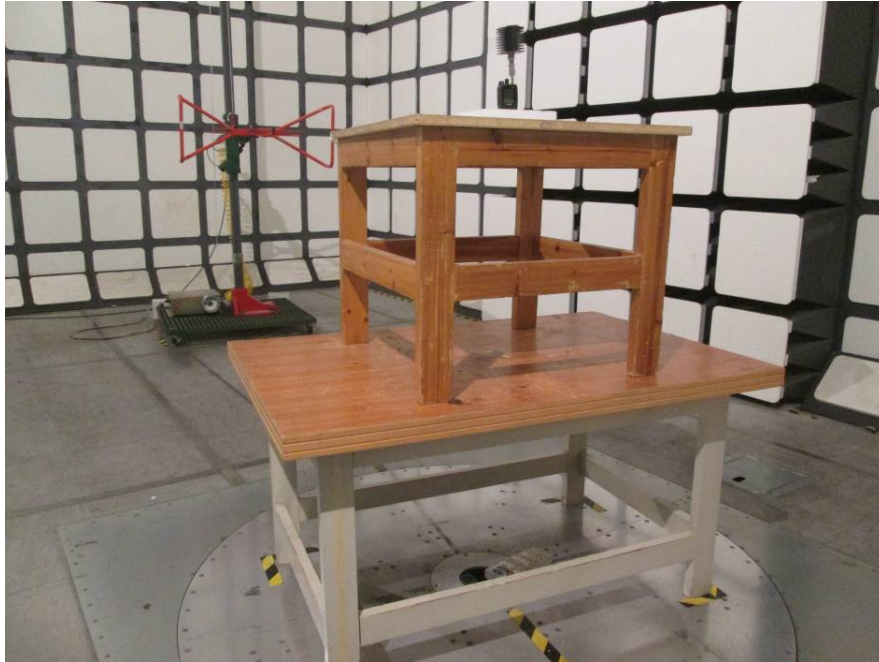
Transmitting Radiated Emissions Tested View (Below 1 GHz)
