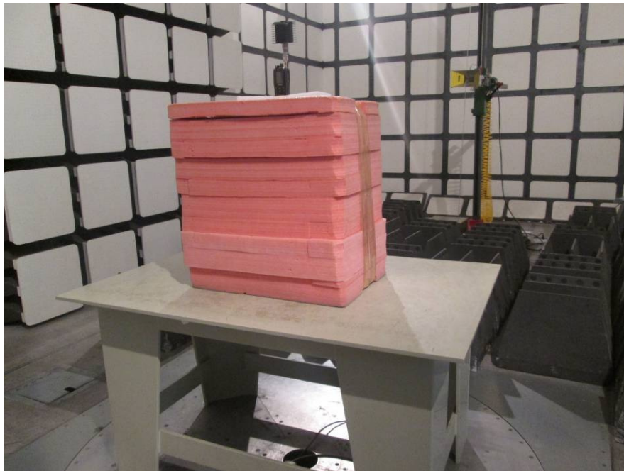
Transmitting Radiated Emissions Tested View (Above 1 GHz)
