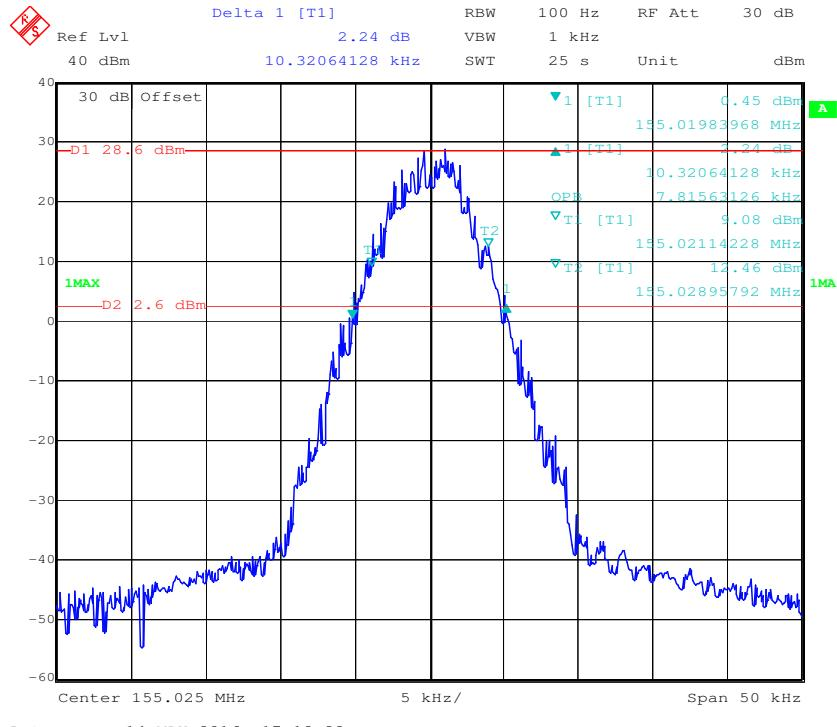
**Frequency 155.025 MHz: 99% Occupied & 26 dB Bandwidth with Low Power**
