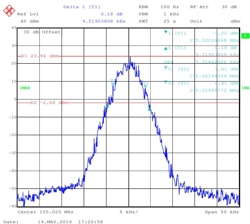
**Frequency 155.025 MHz: Emission Mask, High Power**
