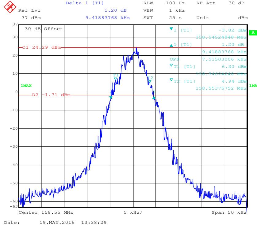
**Frequency 161.025 MHz: 99% Occupied & 26 dB Bandwidth, High Power**
