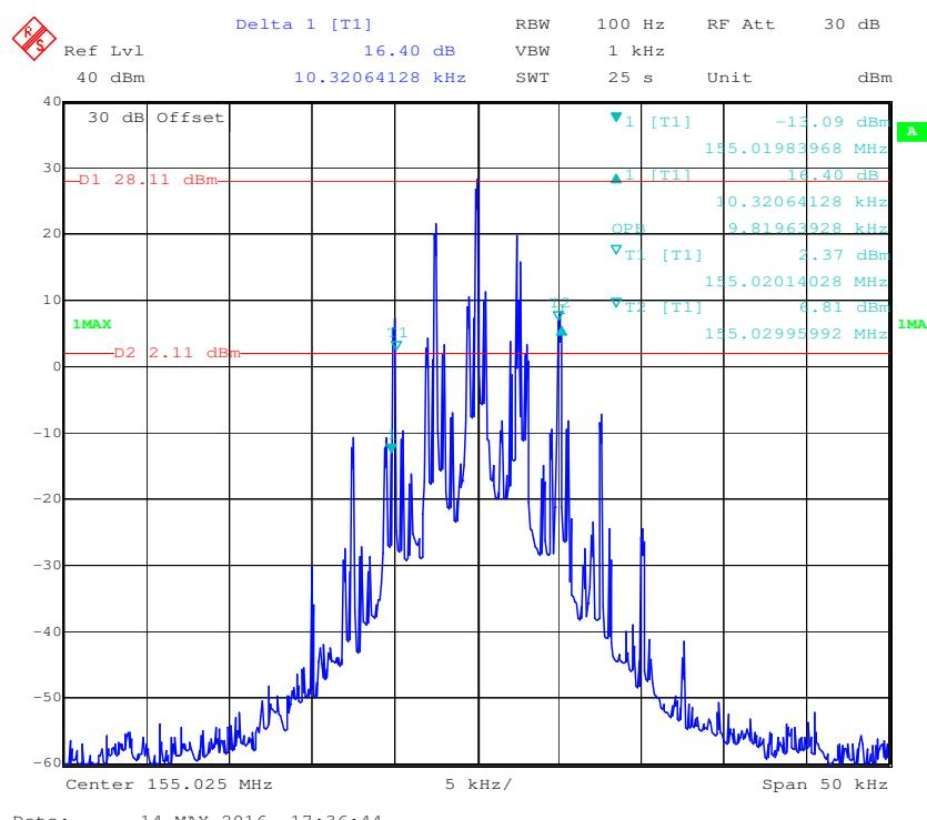
**Frequency 155.025 MHz: Emission Mask, High Power**
