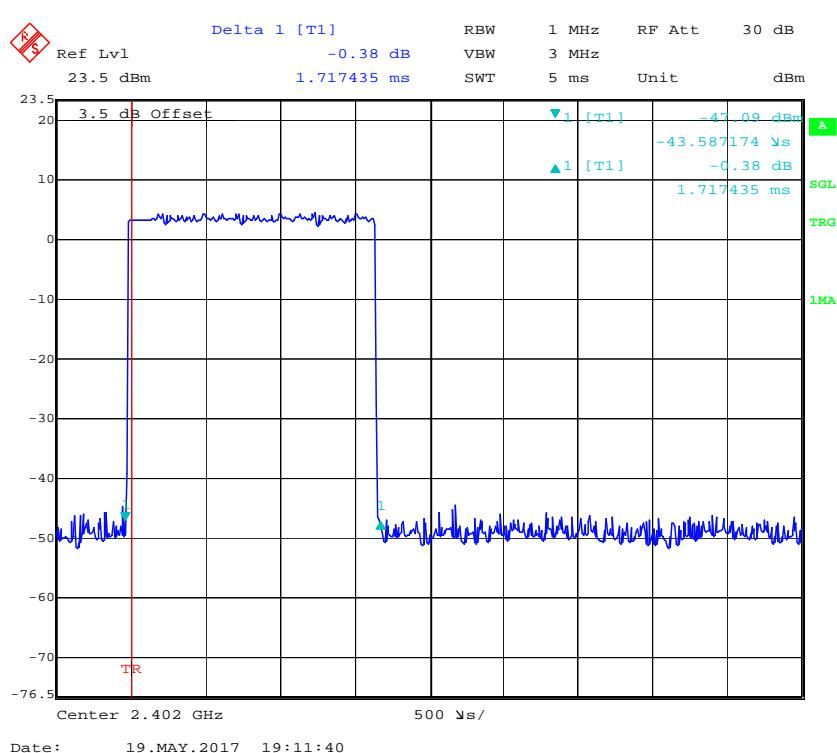
**Pulse time, Middle Channel, 3DH3**
