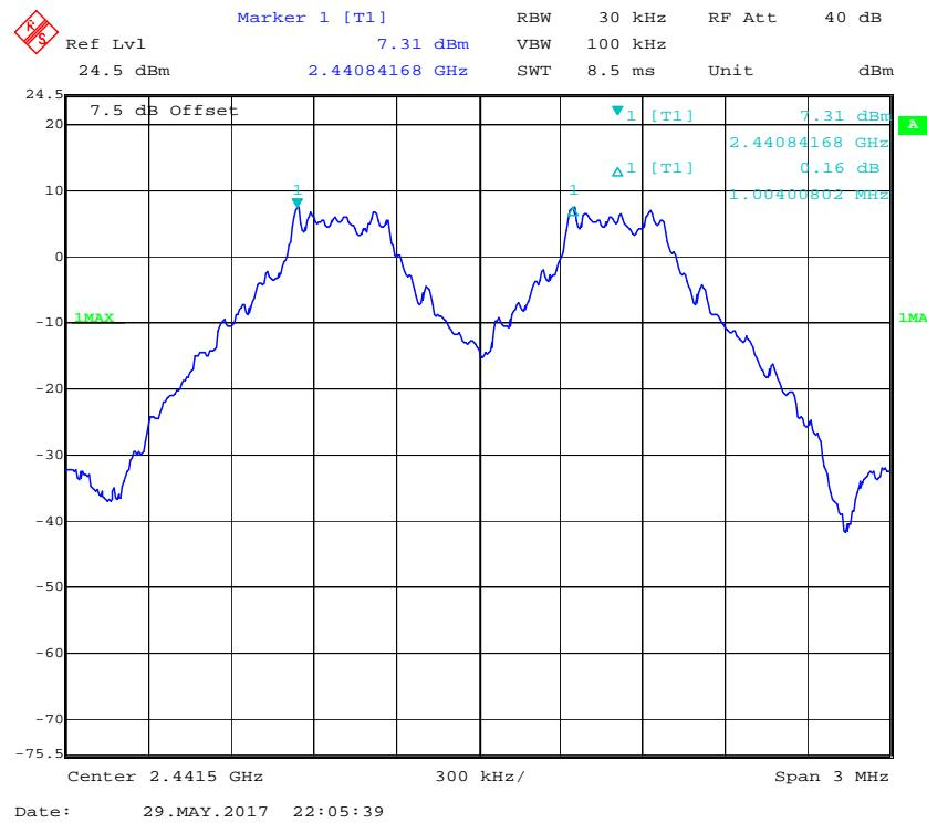
**BDR (GFSK): High Channel**
