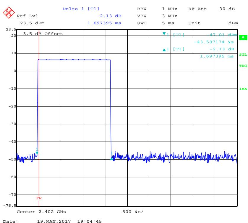
**Pulse time, Middle Channel, DH3**
