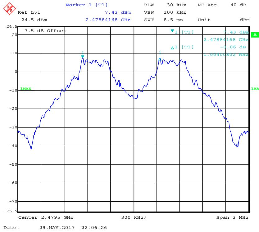
**EDR ( $\pi/4$ -DQPSK): Low Channel**
