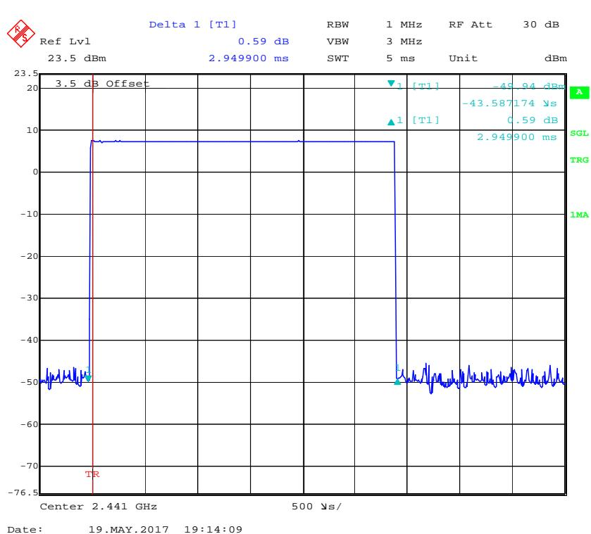
**Pulse time, High Channel, DH5**
