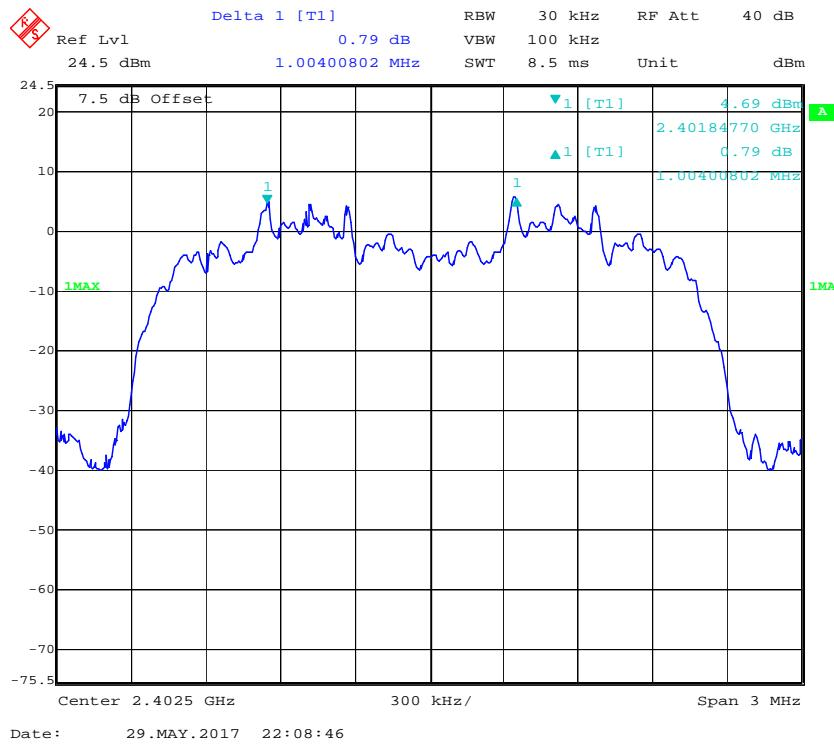
**EDR ( $\pi/4$ -DQPSK): Middle Channel**
