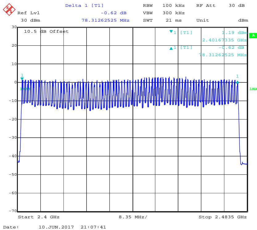
**EDR ( $\pi/4$ -DQPSK): Number of Hopping Channels**
