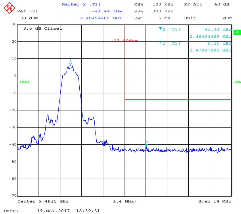
**EDR (8DPSK): Band Edge-Left Side**
