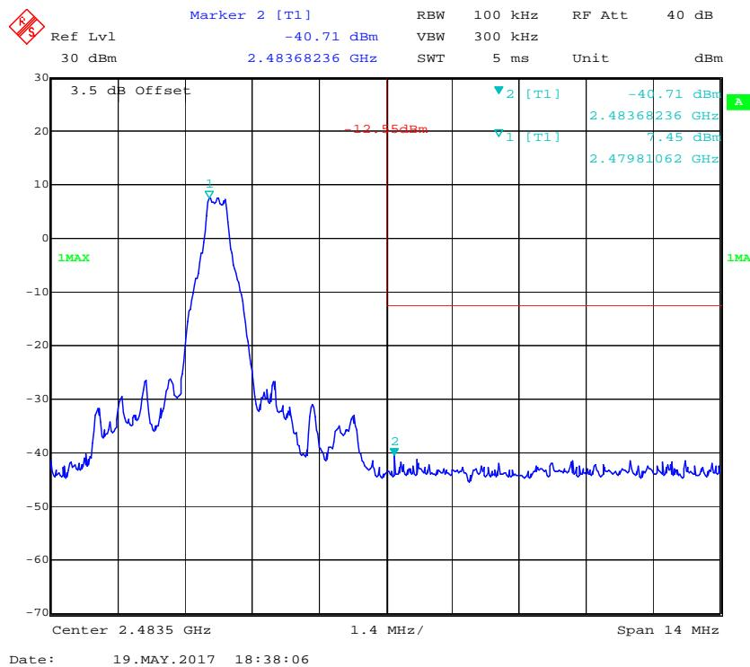
**EDR ( $\pi/4$ -DQPSK): Band Edge-Left Side**
