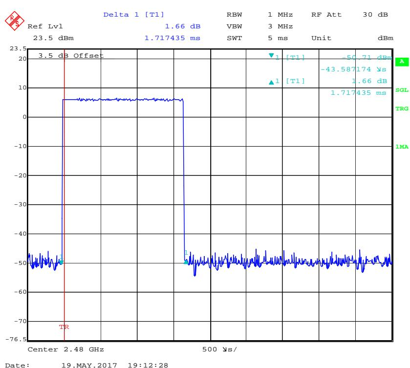
**Pulse time, Low Channel, 3DH5**
