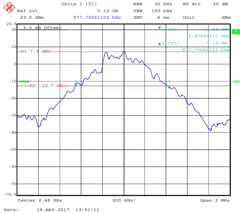
**EDR ( $\pi/4$ -DQPSK): Low Channel**
