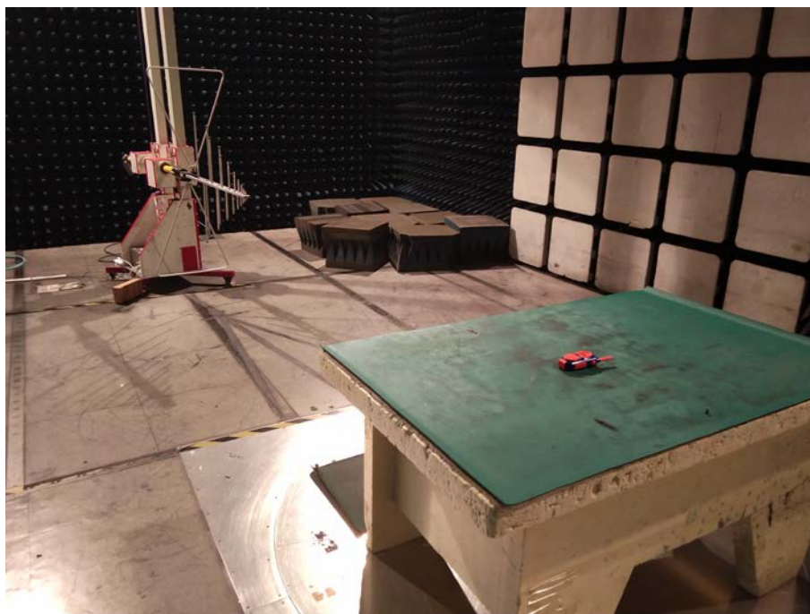
Spurious Emission Test Setup (Below 1GHz)
