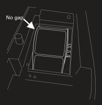
Feed the first label through the label feed guides, making sure the labels are aligned on the left side of the printer.
