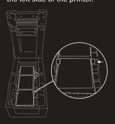
Feed the first label through so it is slightly sticking out of the printer. Then close, plug in, and turn on your GoLabel.
