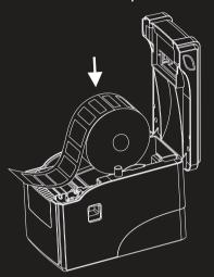
Push the roll of labels to the left so the left side of the roll is flush with the left side of the printer.
