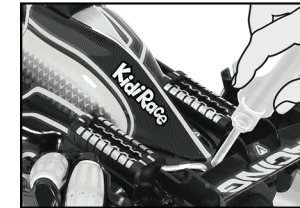
Open the water injection port and fill with clean water.
