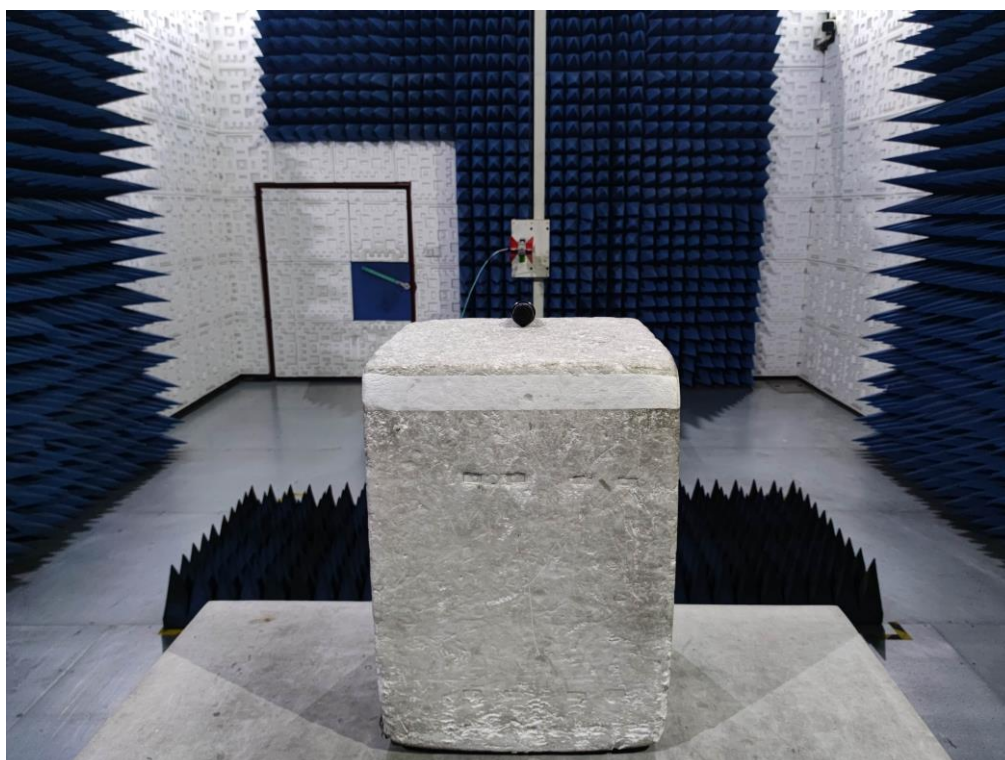
RADIATED EMISSION TEST SETUP ABOVE 1GHz
