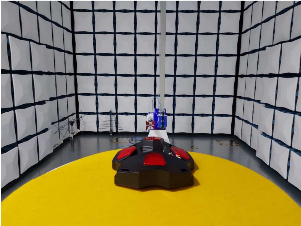
Set-up for Radiated Emission above 1GHz
