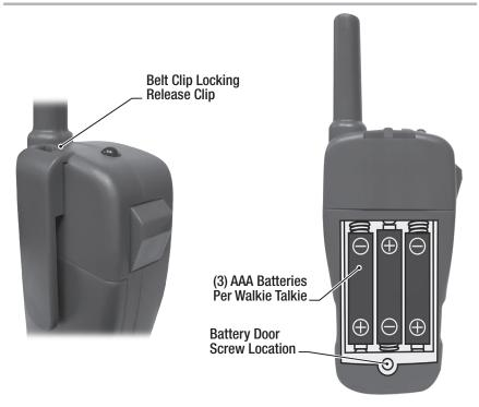
To install the batteries release the belt clip locking clip and slide the belt clip vertically off the back of the walkie talkie body. Remove the battery compartment screw and lift the battery door off. Insert (3) AAA batteries as shown in illustration. Replace battery door and secure with screw. Replace belt clip and ensure it's secure.
