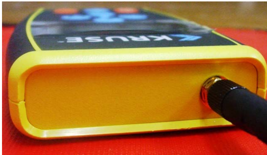
Unique antenna connector – Reverse SMA connector
