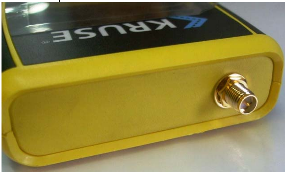
Unique antenna connector – Reverse SMA connector
