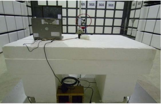
Radiated Emission Set up Photos (Below 1GHz)
