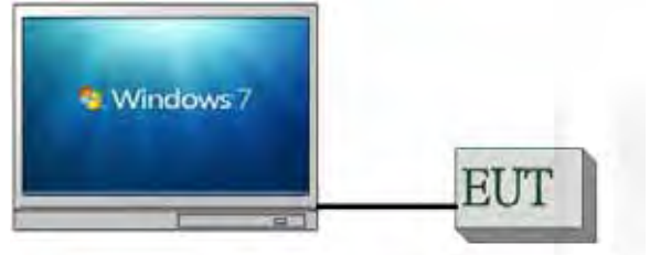
Fig.2-3 Conducted Emission (Antenna Port) Configuration
