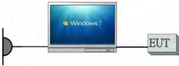
Fig. 2-1 Radiated Emission Configuration
