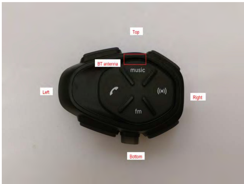
Fig.18 Antenna position of EUT (Front view)
