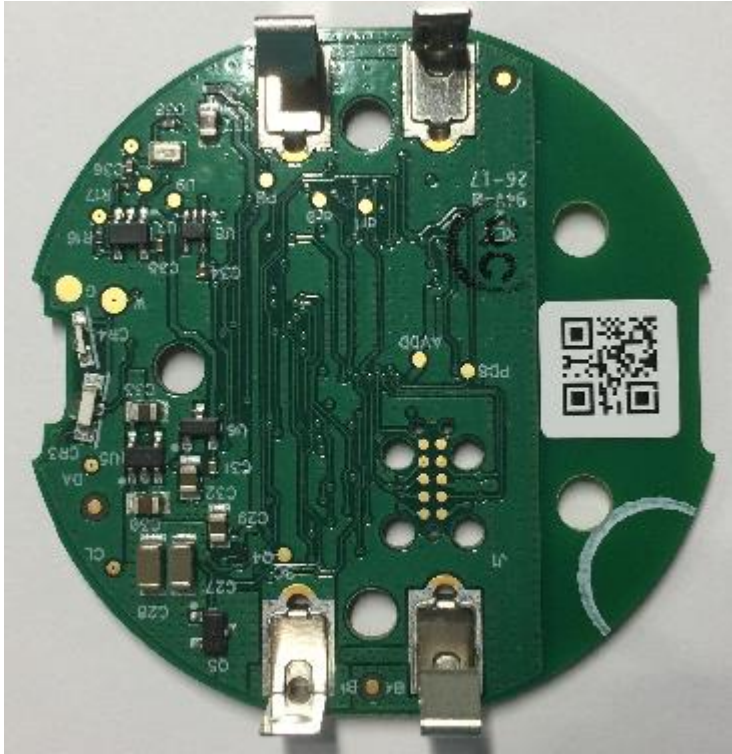
Figure 2- Granite Sensor Model 007, Battery Tab (Bottom) Side
