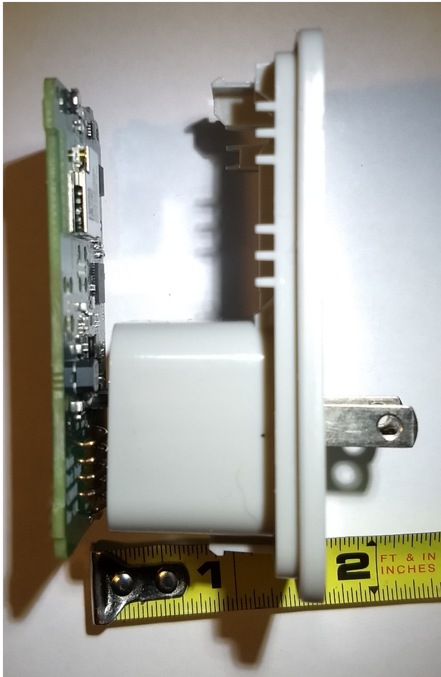
Figure 2, Side View, showing connection to PSU through rear plate of enclosure
