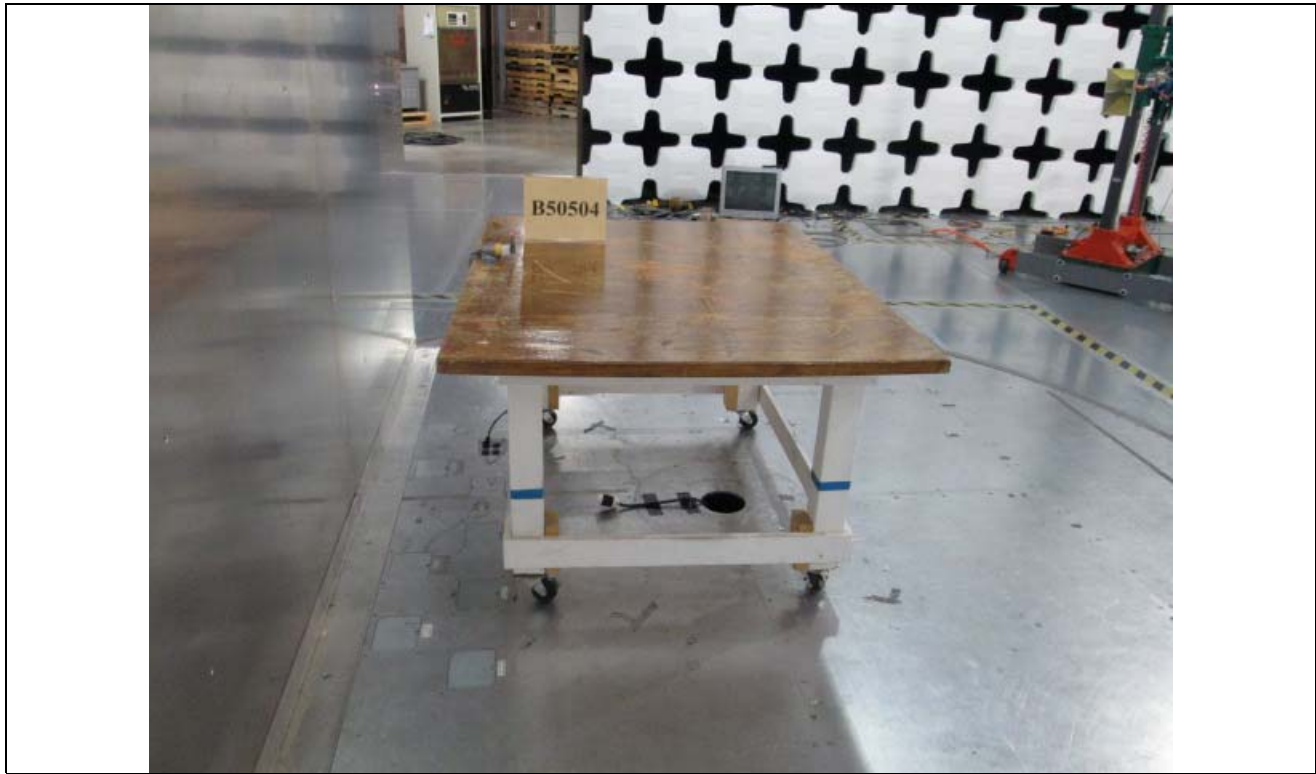
Figure B10: Conducted Emissions Test Setup - Left
