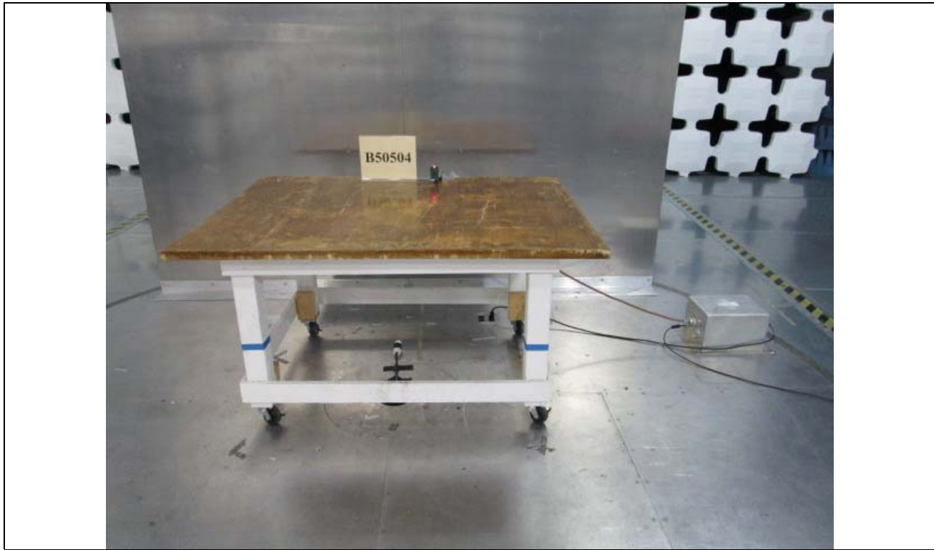
Figure B7: Conducted Emissions Test Setup - Front
