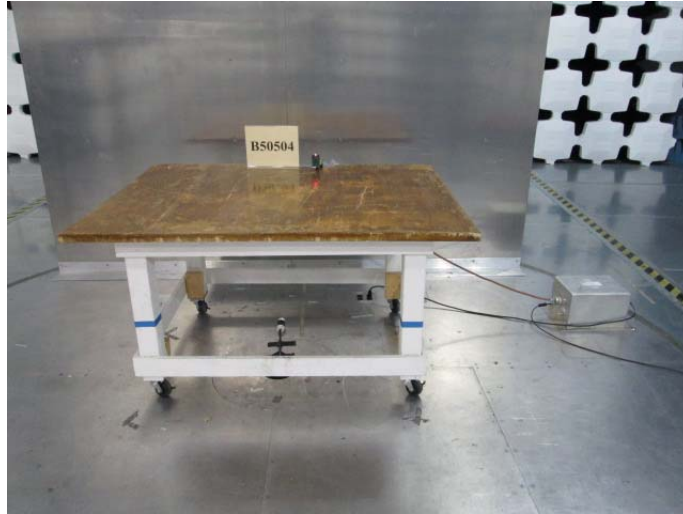
Test Setup – Conducted Measurements – AC Mains
