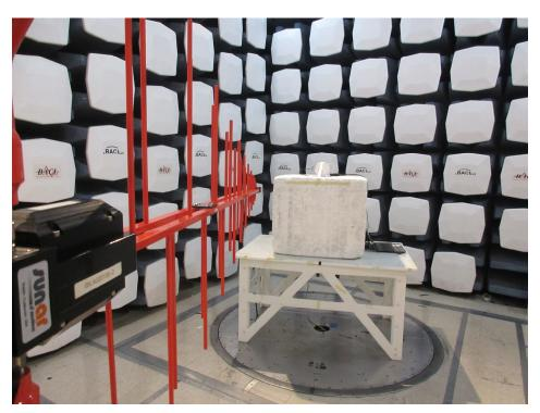
1.2 Radiated Emission below 1 GHz Rear View
