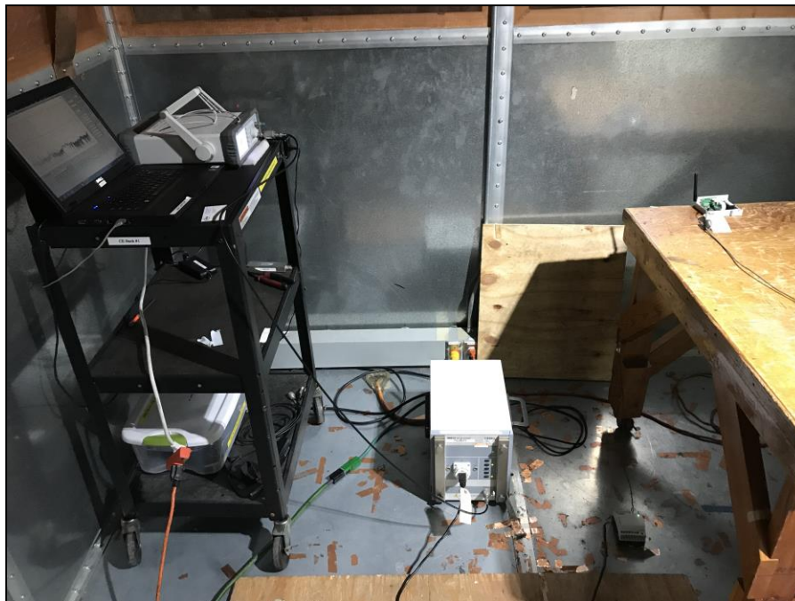
Photograph 2. Conducted Emissions, 15.207(a), Test Setup
