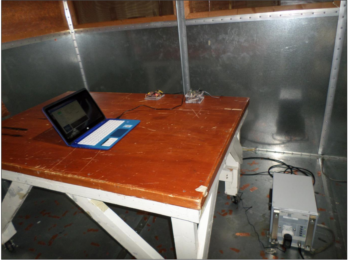
Photograph 1. Conducted Emissions, 15.207(a), Test Setup
