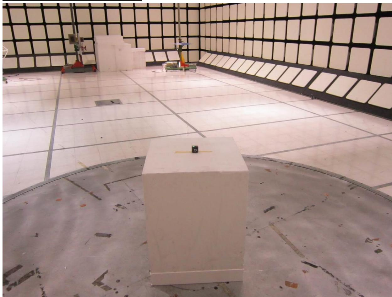
\* similar setup used for 9kHz-30MHz but the loop antenna would be in the middle of the room, 3m away from the EUT.
