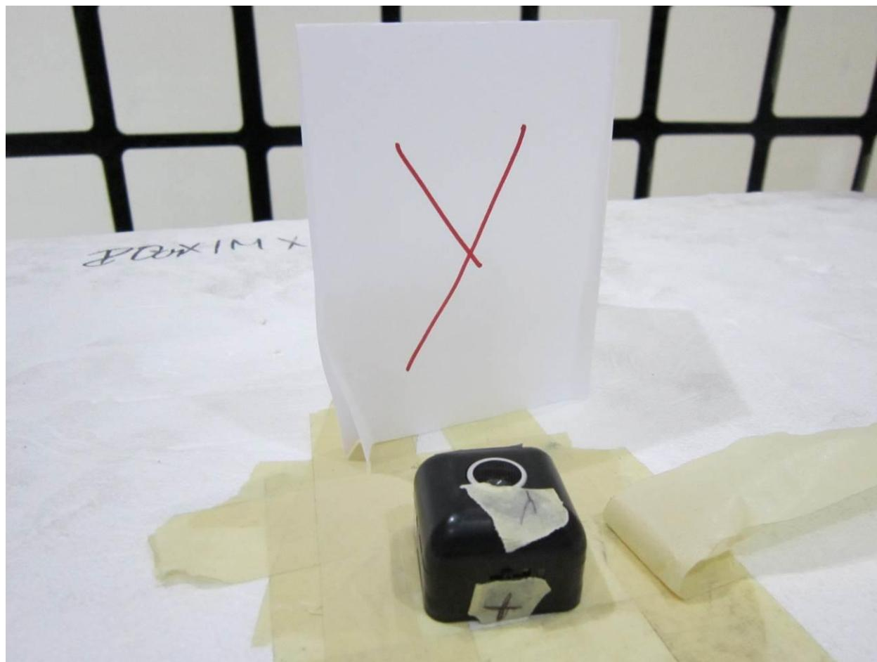
**Z-Axis Setup for Radiated Emissions**
