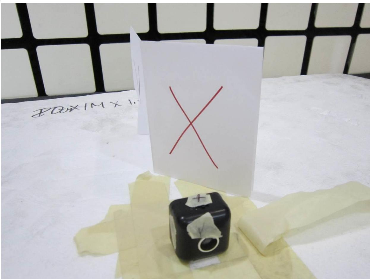
**Y-Axis Setup for Radiated Emissions**
