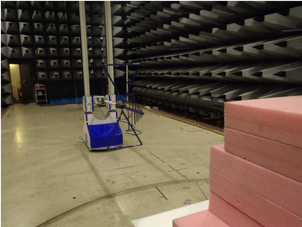
Photo 4.2.2 Test setup regarding measurement of radiated emission.
