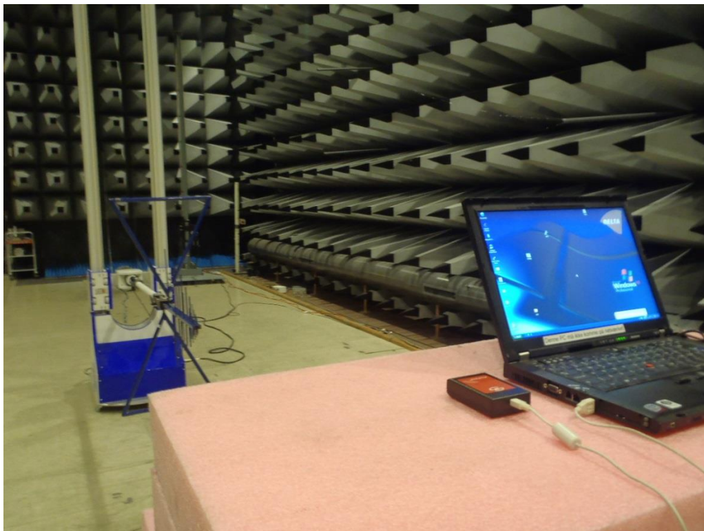
Photo.4.3.1 Test setup regarding measurement of field strength of fundamental.
