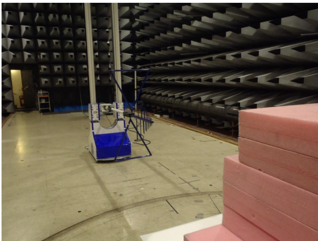
Photo 4.3.2 Test setup regarding measurement of field strength of fundamental.
