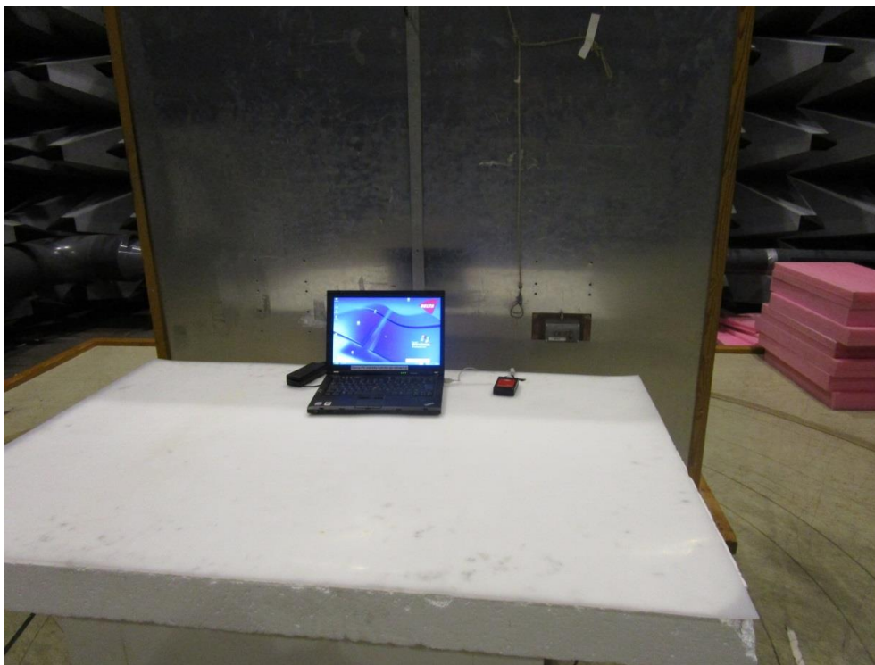
Photo 4.1.1 Test setup regarding measurement of radio frequency voltage on mains.
