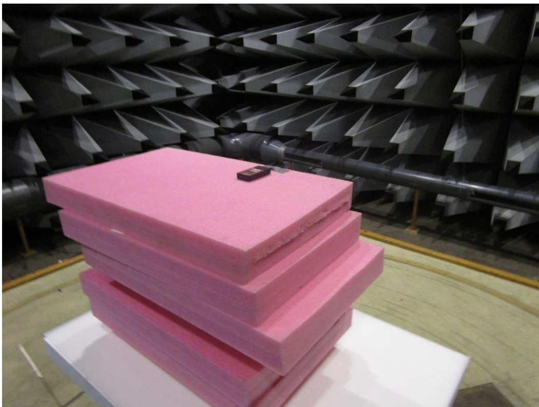
Photo 4.2.2 Test setup regarding measurement of field strength of fundamental.
