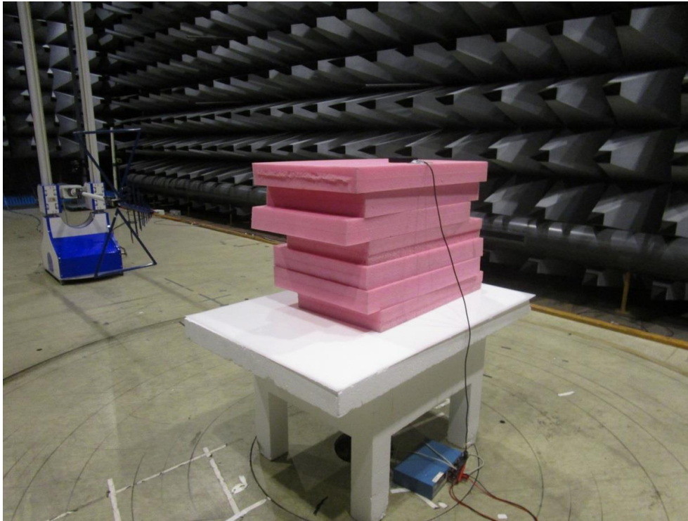
Photo 4.1.1 Test setup regarding measurement of radiated emission.
