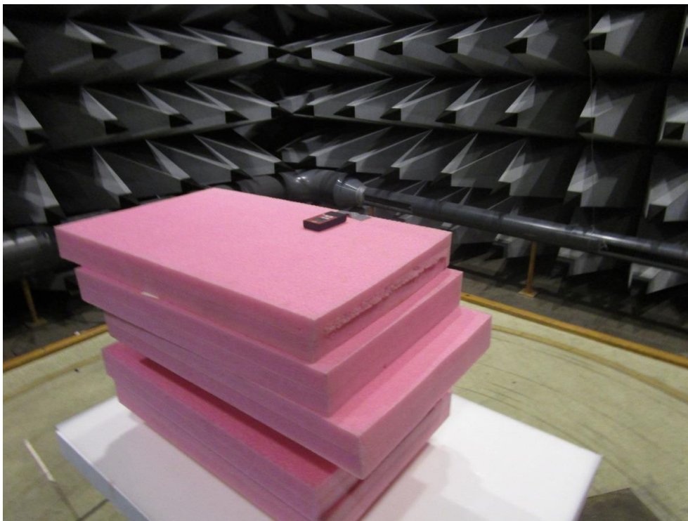
Photo 4.1.2 Test setup regarding measurement of radiated emission.
