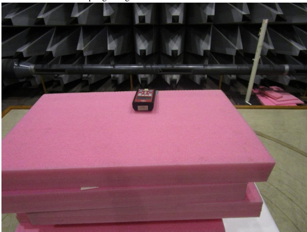
Photo 4.1.2 Test setup regarding measurement of radiated emission.
