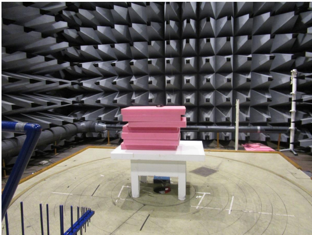
Photo 4.1.1 Test setup regarding measurement of radiated emission.
