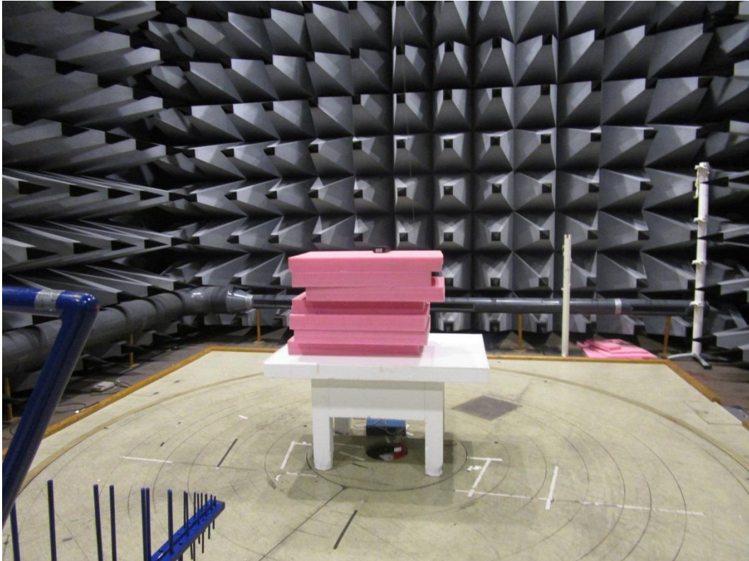
Photo 4.2.1 Test setup regarding measurement of field strength of fundamental.
