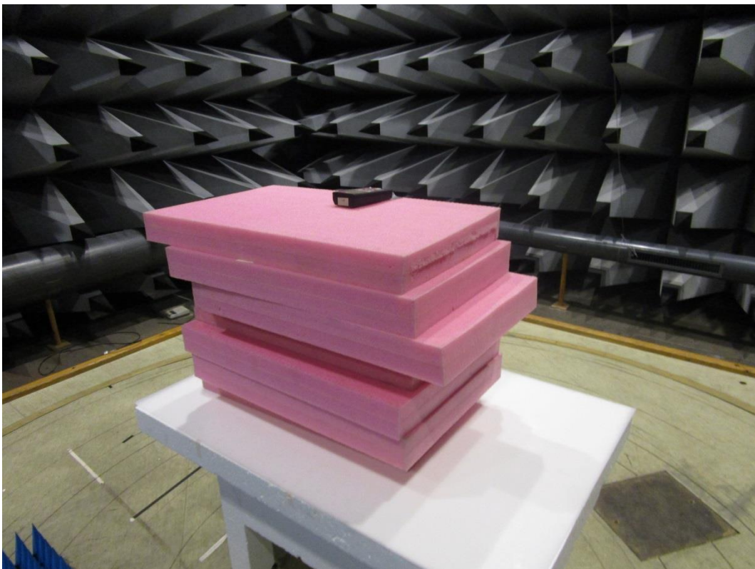
Photo 4.1.4 Test setup regarding measurement of radiated emission.
