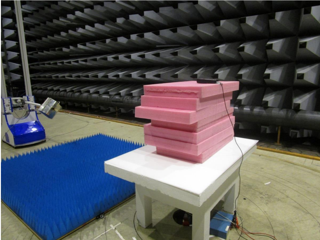
Photo 4.1.3 Test setup regarding measurement of radiated emission.
