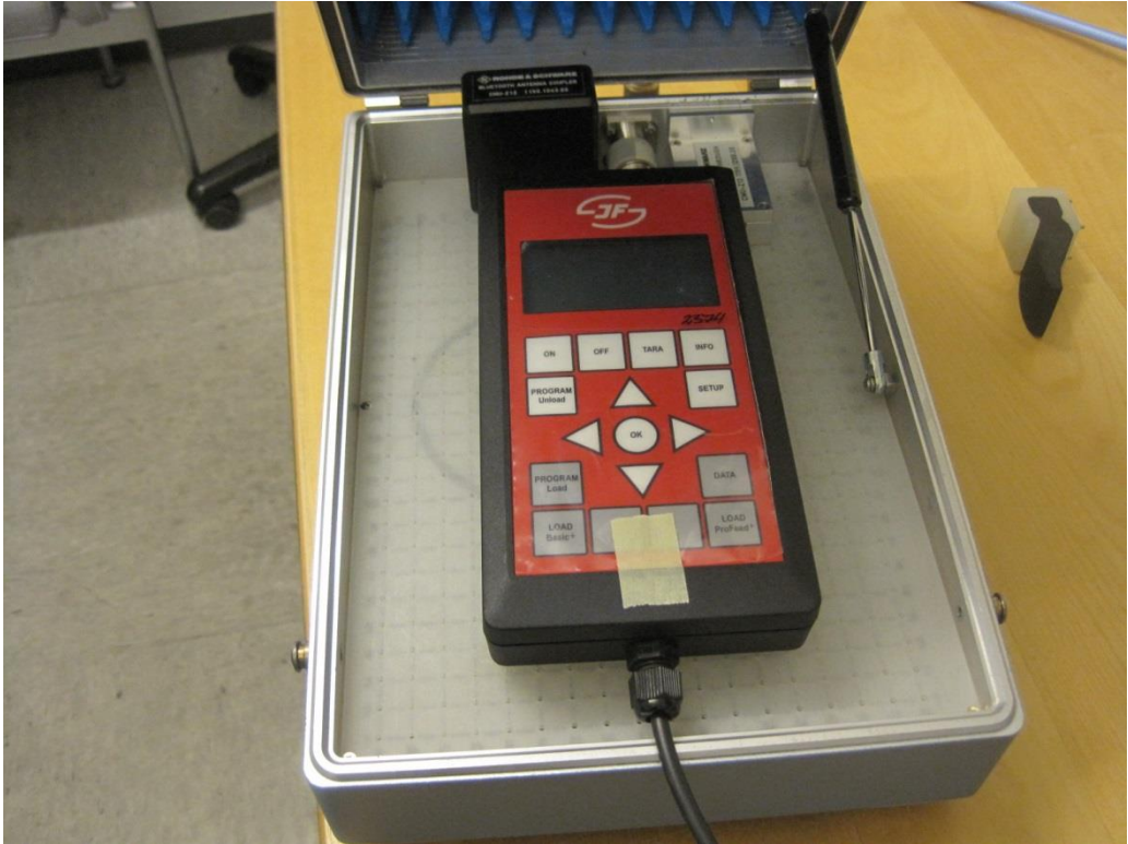
Photo 4.4.1 Test setup regarding measurement of 20 dB bandwidth.
