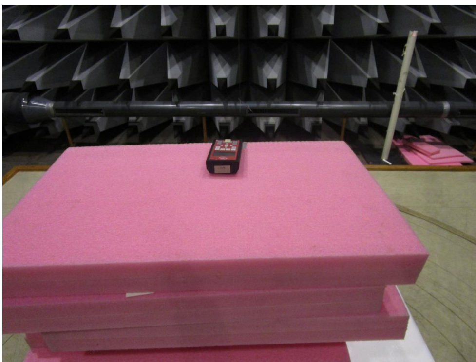
Photo 4.2.2 Test setup regarding measurement of field strength of fundamental.
