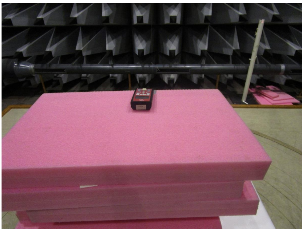
Photo 4.1.2 Test setup regarding measurement of radiated emission.
