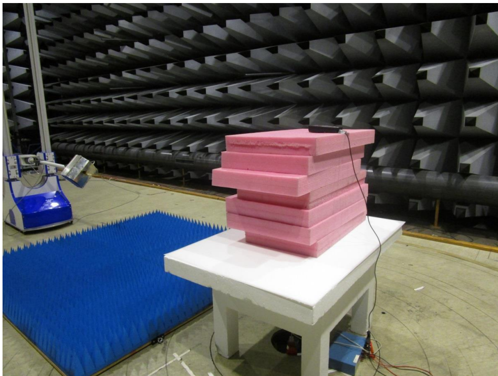
Photo 4.1.3 Test setup regarding measurement of radiated emission.
