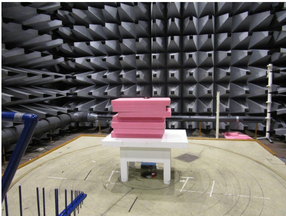
Photo 4.1.1 Test setup regarding measurement of radiated emission.
