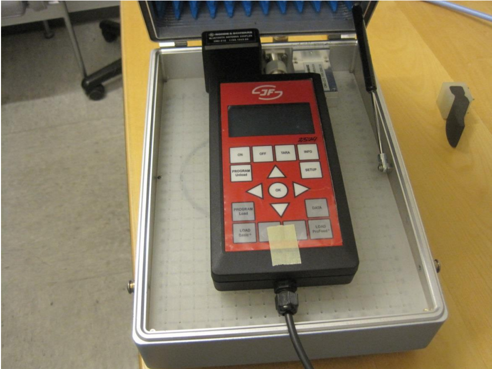
Photo 4.4.1 Test setup regarding measurement of 20 dB bandwidth.
