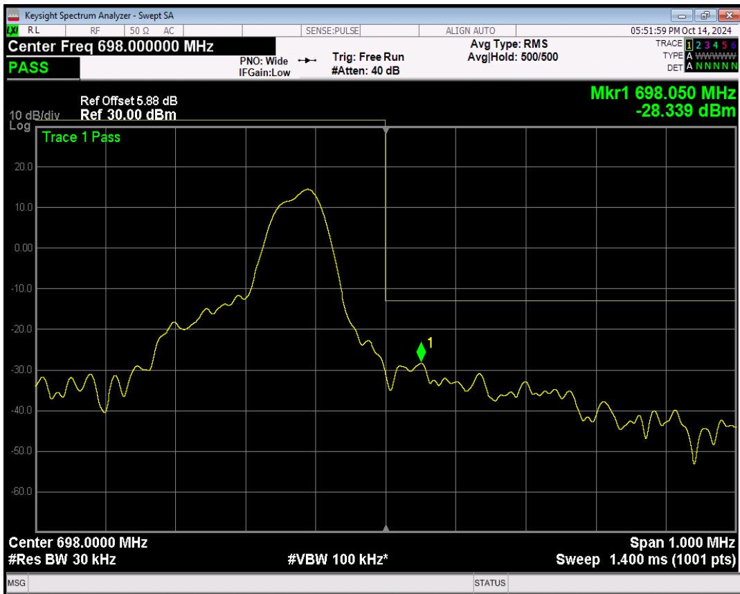
Band71 BPSK Channel=133470 nTones=1@11 Spacing=15kHz
