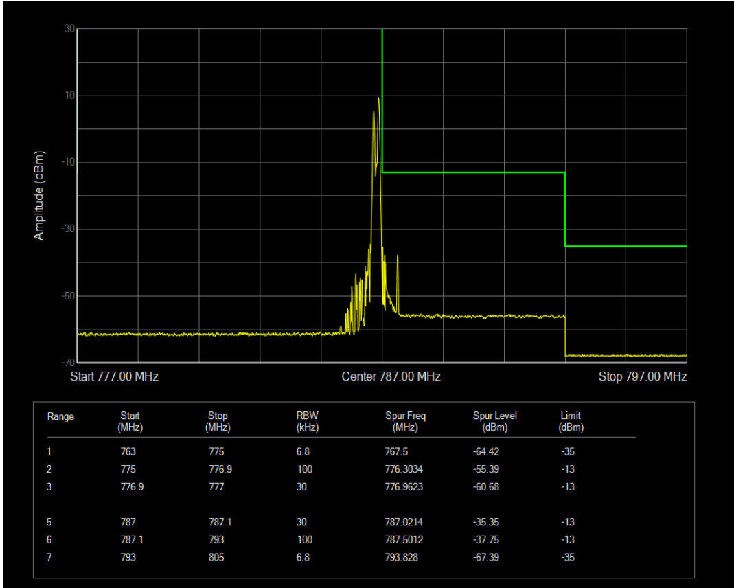
Band13 QPSK Channel=23278 nTones=1@11 Spacing=15kHz
