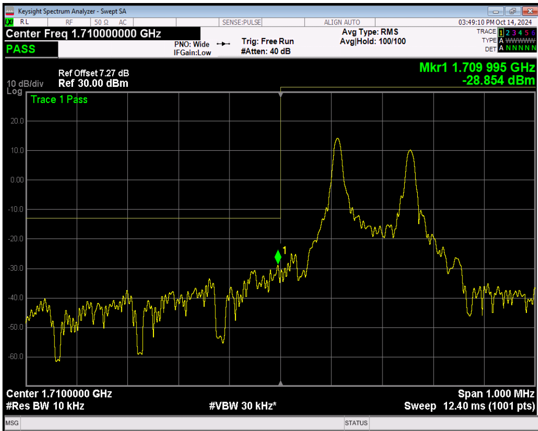
Band66 QPSK Channel=131974 nTones=1@0 Spacing=3.75kHz
