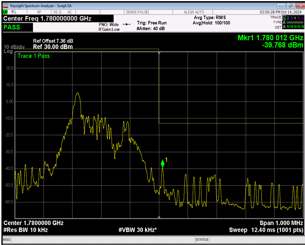
Band71 BPSK Channel=133124 nTones=1@0 Spacing=3.75kHz
