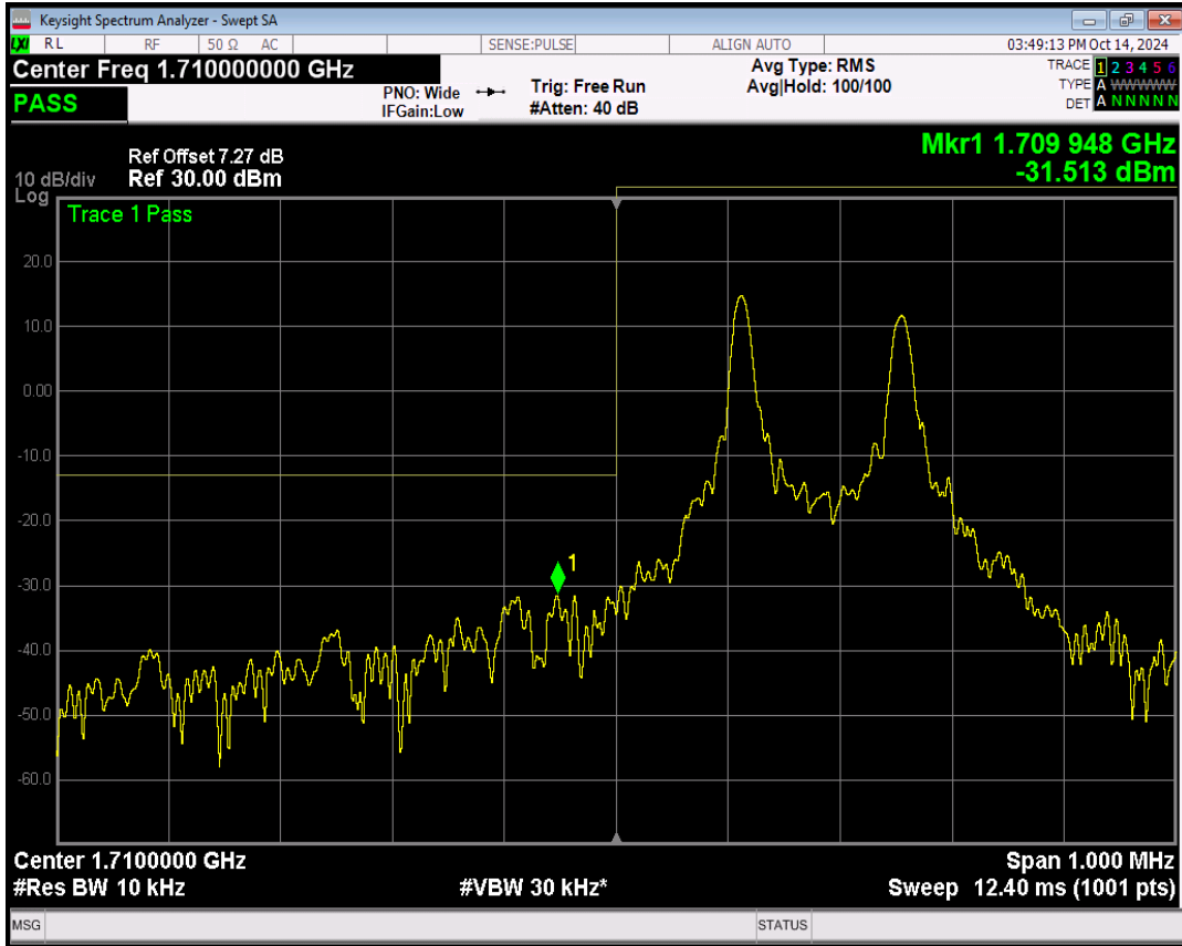
Band66 BPSK Channel=131974 nTones=1@0 Spacing=15kHz
