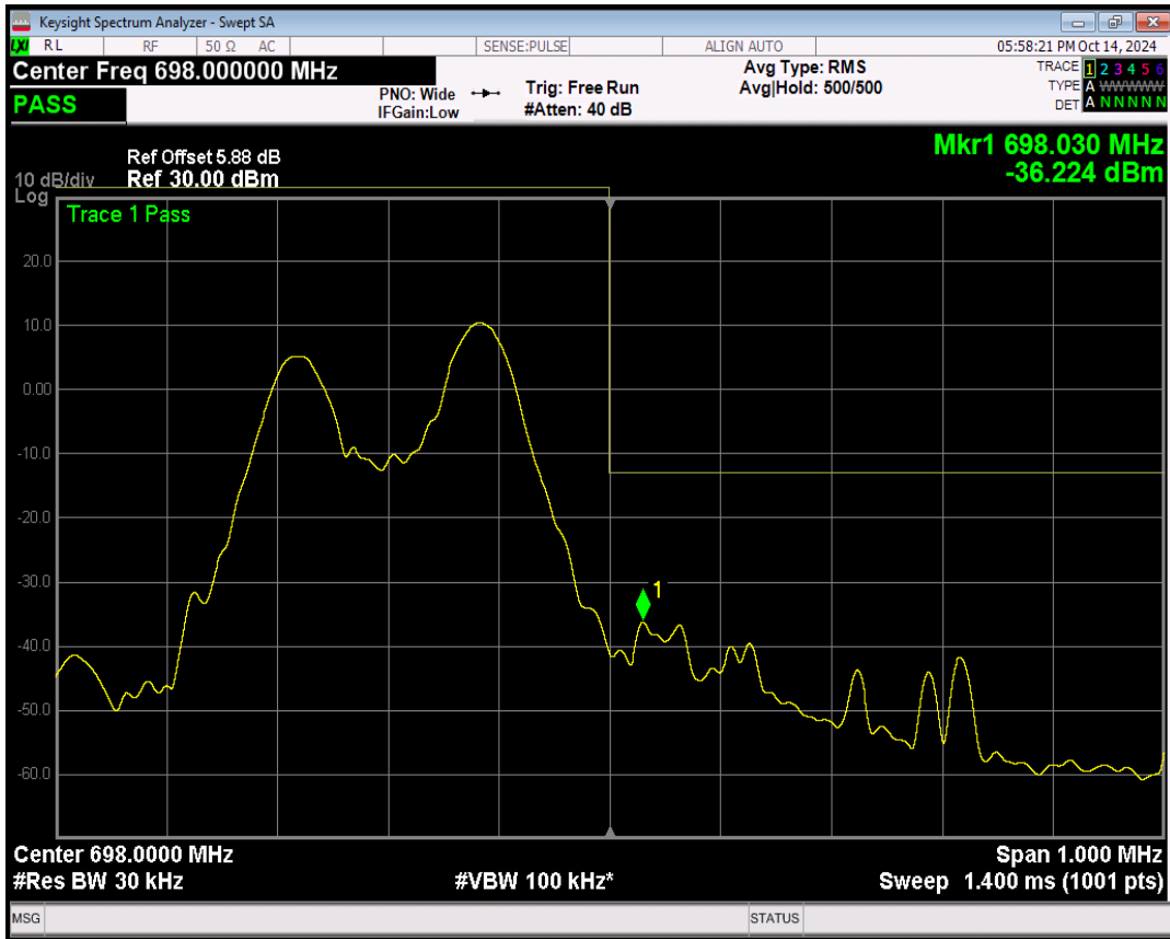
Band71 QPSK Channel=133470 nTones=1@11 Spacing=15kHz
