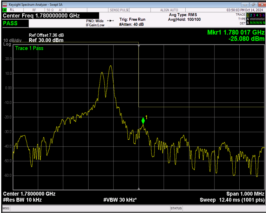
Band66 QPSK Channel=132670 nTones=1@47 Spacing=3.75kHz
