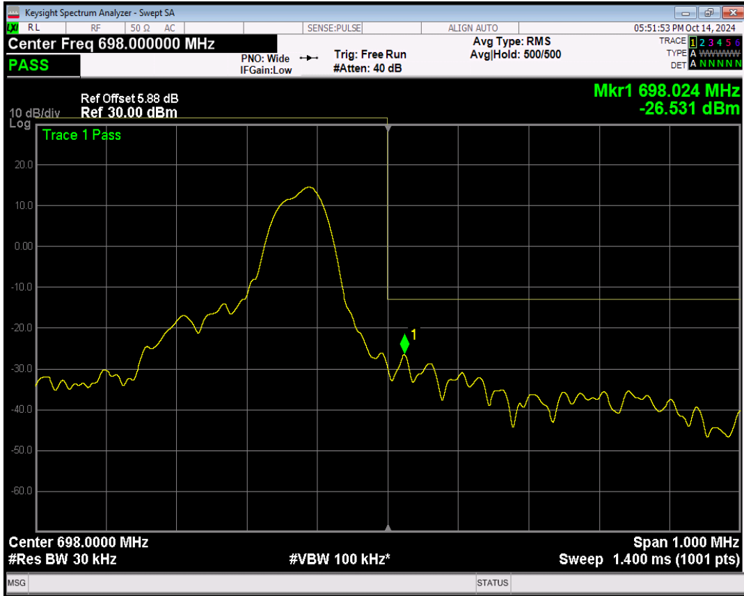
Band71 QPSK Channel=133470 nTones=1@47 Spacing=3.75kHz
