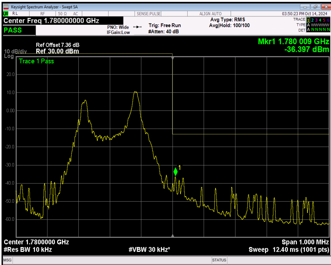
Band66 QPSK Channel=132670 nTones=12@0 Spacing=15kHz
