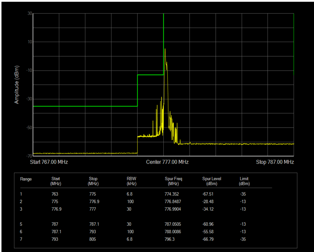
Band13 BPSK Channel=23278 nTones=1@47 Spacing=3.75kHz
