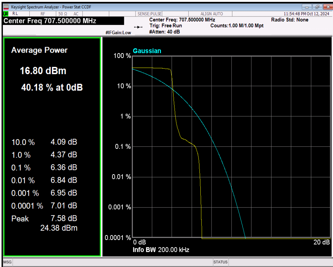
Band12 QPSK Channel=23095 nTones=1@0 Spacing=3.75kHz
