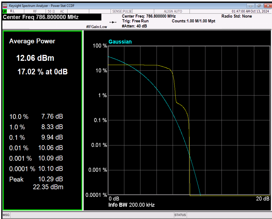
Band13 QPSK Channel=23278 nTones=1@0 Spacing=15kHz
