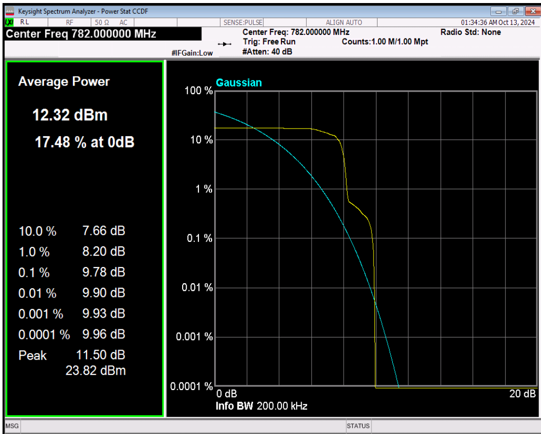
Band13 QPSK Channel=23230 nTones=1@0 Spacing=15kHz
