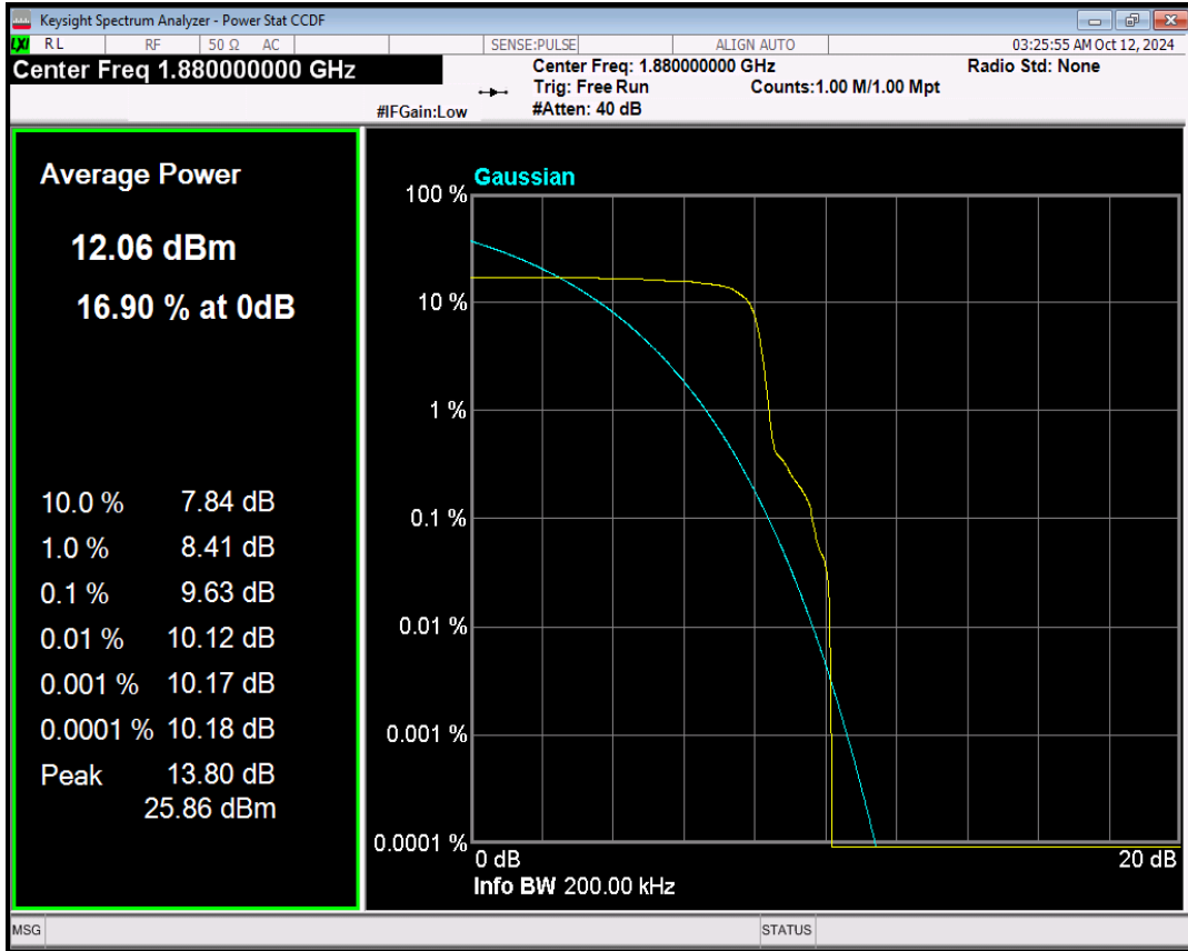
Band2 QPSK Channel=19198 nTones=1@0 Spacing=3.75kHz
