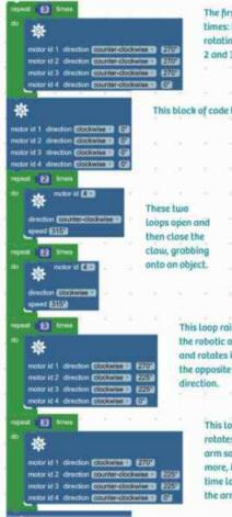
The first loop repeats the following three times: It turns motor 1 counterclockwise, rotating the robatic arm; and it turns motors 2 and 3 counterclockwise, lowering the arm.
