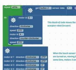
The first part of the program is a loop which repeats as long as the touch sensor has not been activated.
