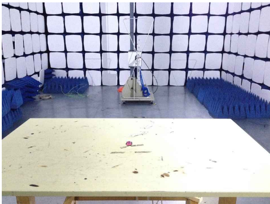
Radiation Emission Test Setup (30MHz to 1GHz)
