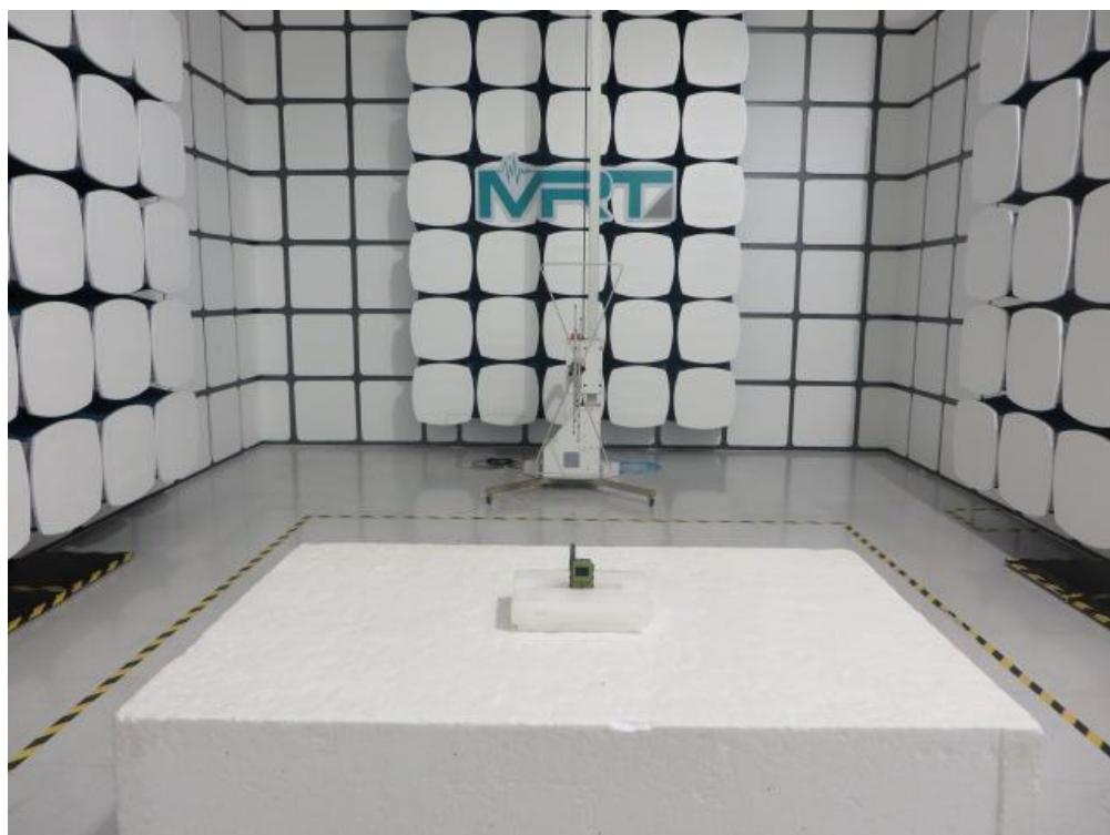
Description: Radiated Emission Test Setup for 1GHz ~ 5GHz
