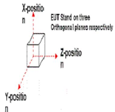
Note: We test X-axis, Y-axis, and Z-axis,. The Y-axis is the worst mode, so only the worst mode test data was included in the report.
