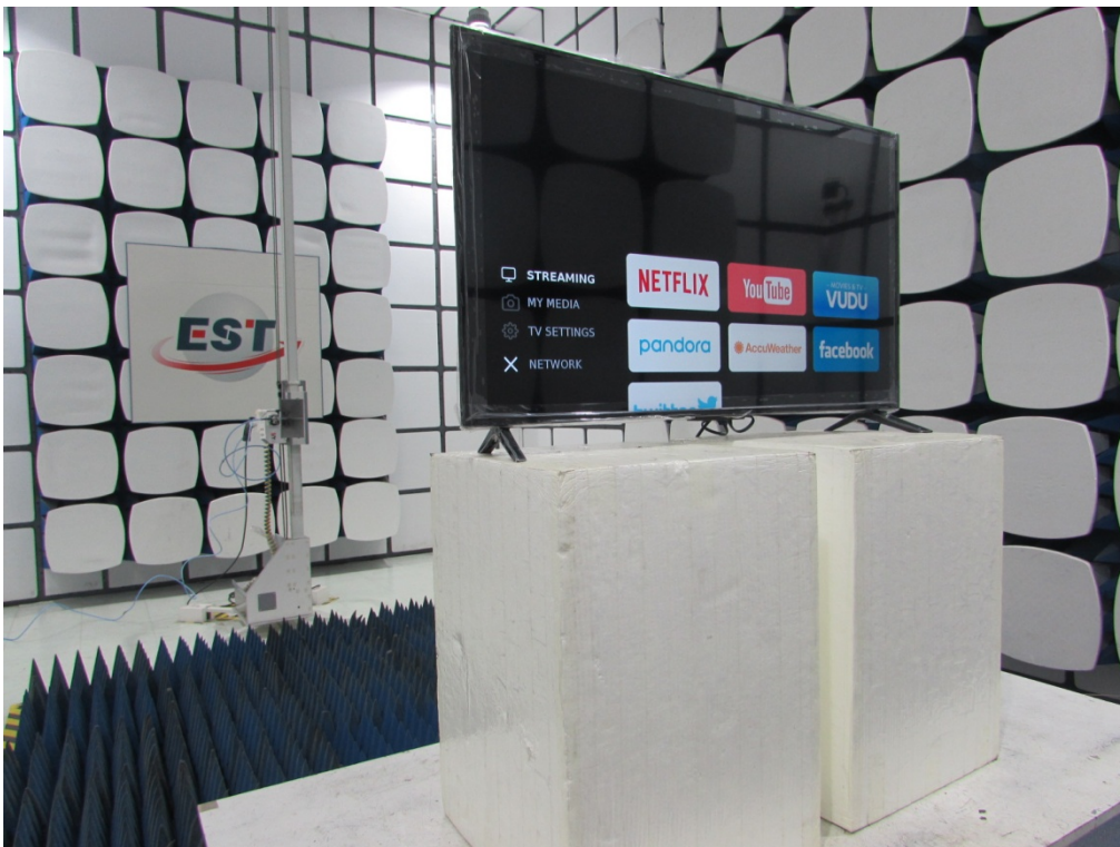
Radiated Test (Above 1000 MHz)
