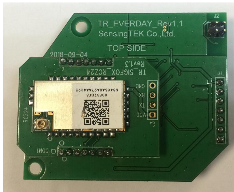
Fig.5 Module_Sigfox_RCZ2 hardware installation diagram
