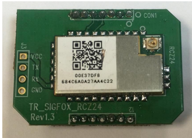
Fig.4 Module_Sigfox_RCZ2 on the carrier board
