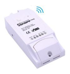
onoff TH10/16 is a Sonoff version that can monitor and set temperature and humidity through the APP eWeLink. Just as the name indicats, the new version Sonoff TH device supports two power supply specifications: 10A or 16A. Sonoff TH 10/16 supports presetting range for temperature or humidity, when the temperature or humidity of the environment falls into the range, it will automatically turn on or turn off connected devices.
