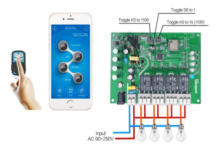
2. In inching mode, you can turn on the connected devices for 0.25-4s. For example, you can turn on CH1 connected device for 1s, then auto-off.
