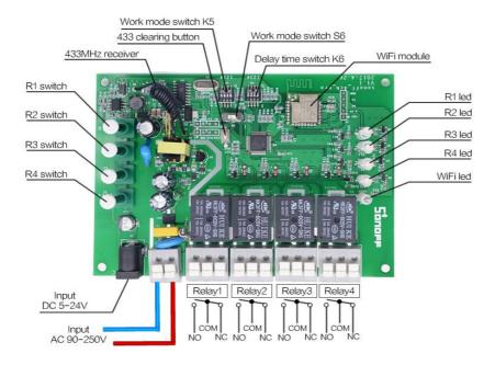
You may choose to power up by 5-24V DC or by 90-250V AC. Each relay without voltage output.
