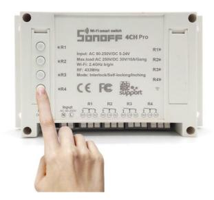
$2.\ Press\ and\ hold\ one\ of\ the\ 4\ ON/OFF\ buttons\ for\ 7\ seconds\ until\ the\ wifi\ LED\ fast\ blinks\ 3\ times\ and\ repeat.$
