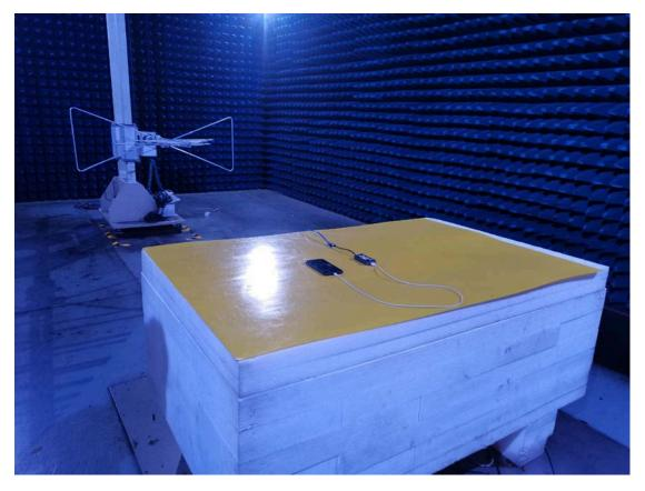
Photo of Radiated Emission Measurement Above 1GHz
